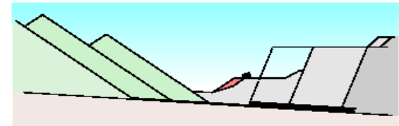
1. The overburden is blasted with moderate throw, then dozed to form the dragline bench
